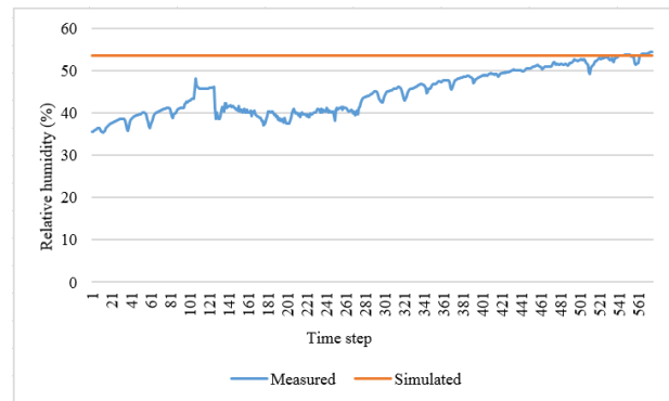
Figure 20: Monitored and simulated Relative humidity values of Hempod.
