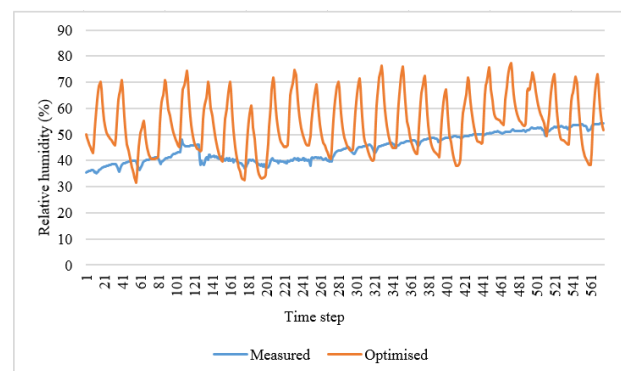
Figure 18: Monitored and optimised Relative humidity values of Hemm.
