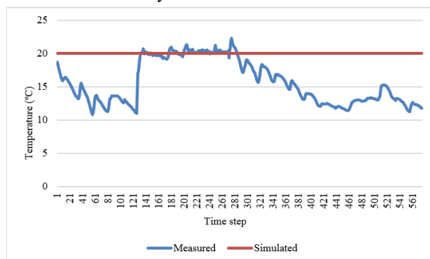
Figure 19: Monitored and simulated temperature values of Hempod.
